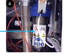
Remove the filter and disassemble the blue armature core (by unscrewing the removable cap) to re-use on the new element.
