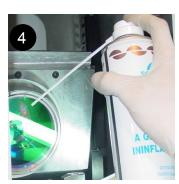
7. Soak slightly an optical paper towel in optical cleaning fluid.
