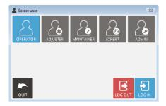
Operator level: first user level including a printer preparation wizard, showing the step-by-step instructions on how to prepare/to start a job and to remove the built part when job complete.
