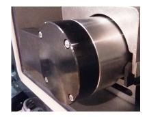
The combination of different movements of roller and carriage are adjustable for carrying out actions of layering such as spreading, smoothing and compacting. The layer thickness of powder differs depending on the material properties (particle size, flowability...) and on the desired part characteristics.
