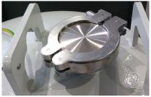
Step c : clamp tightening
