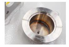
• Install the centering ring with standoff tube in the filter outlet port. The stem of the centering ring must be placed directly on the locating pin of the internal valve.
