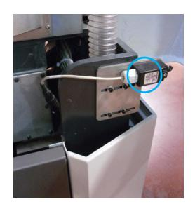
Safety interlock switch on the scanner head
