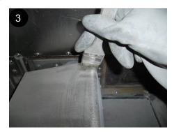
4. Move the carriage up to the sintering piston, then clean the left side of the manufacturing chamber (4), sweeping the powder toward the collecting cans.
