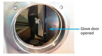
• To close the glove door, make sure the Flat Bar is placed at first vertically. Then fully close the glove door, and place the Flat Bar horizontally (as shown on the left figure). Make sure to tighten securily the Palm Grip while the Flat Bar is placed horizontally.
