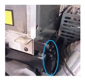
Safety interlock switch on the airlock door
